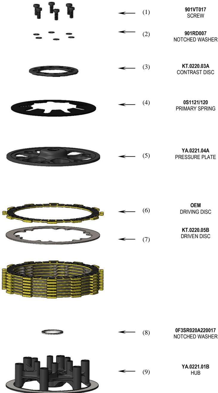
The operation of the clutch is closely related to the height of the disc pack. It is therefore necessary to measure the disc pack before mounting. From the original clutch take only the driving discs, then assemble the disc pack using the driven discs (7) supplied in the package and take the measurement.
