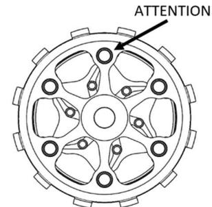
Position the primary spring (3) in the seat on the pressure plate (4). Then install the contrast disc (2) keeping the code writing visible to the operator.
