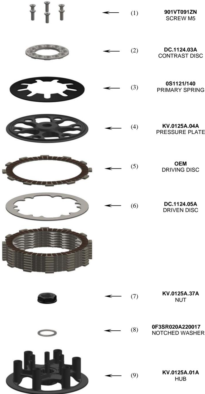
The operation of the clutch is closely related to the height of the disc pack. It is therefore necessary to measure the discs set before mounting. From the original clutch take only the driving discs, then assemble the disc pack using the driven discs (6) supplied in the package and take the measurement. The total height of the disc pack must be equal to **32.9 ± 0.2 mm**.
