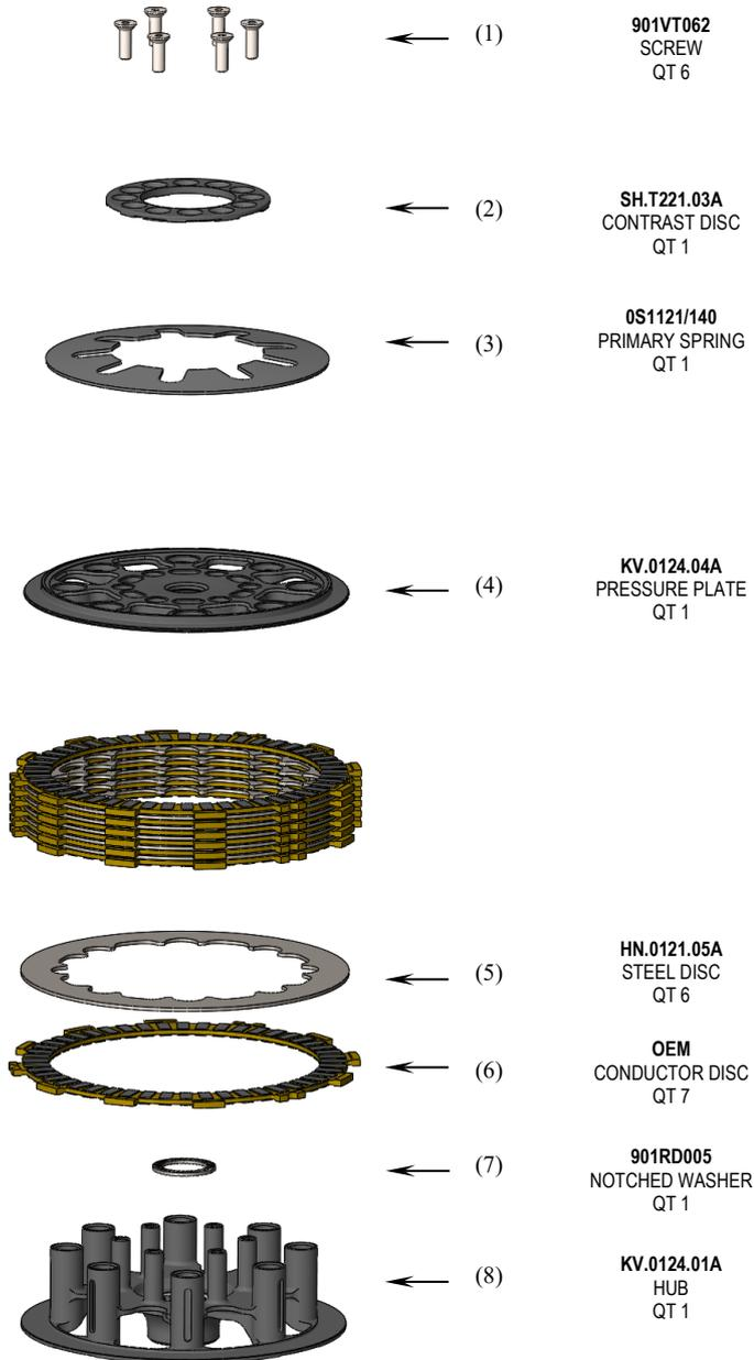
**The assembly procedure must be carried out by specialized personnel.** The operation of the clutch is strictly related to the height of the disc pack. It is therefore necessary to measure the disc pack before assembly. From the original clutch, take only the driving discs, then assemble the disc pack using the driven discs (5) supplied in the package and carry out the measurement.
