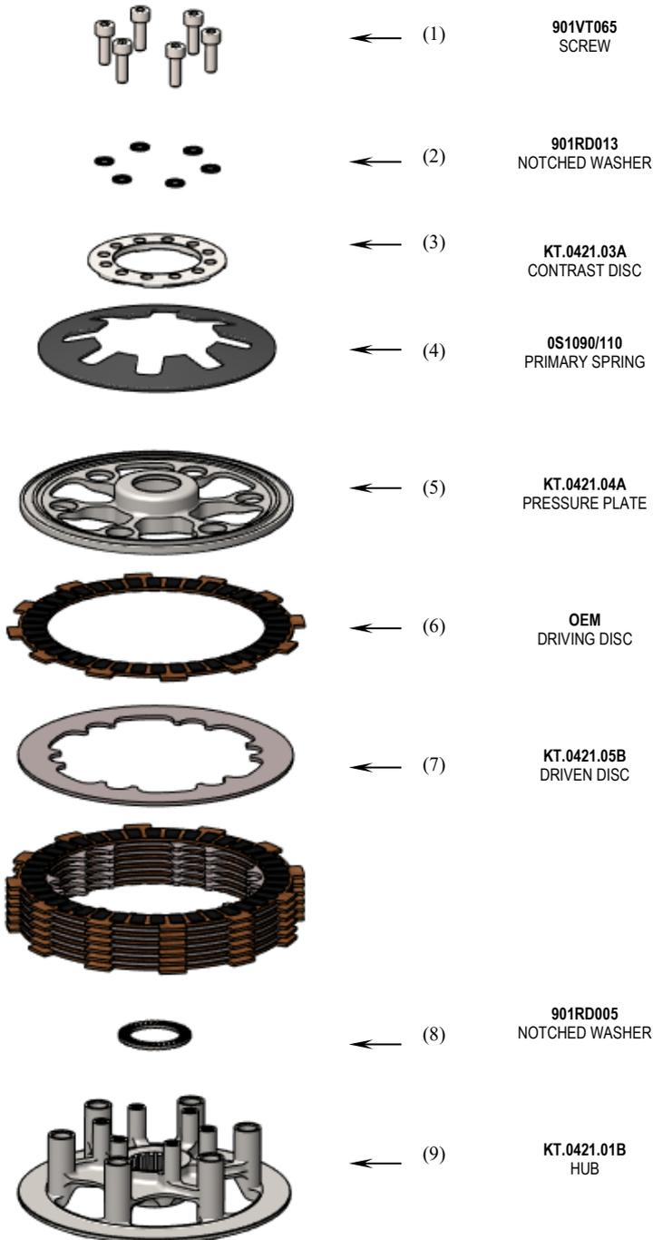
The operation of the clutch is closely related to the height of the disc set. It is therefore necessary to measure the disc set before mounting. From the original clutch take only the driving discs, then assemble the disc set using the driven discs (7) supplied in the package and take the measurement.
