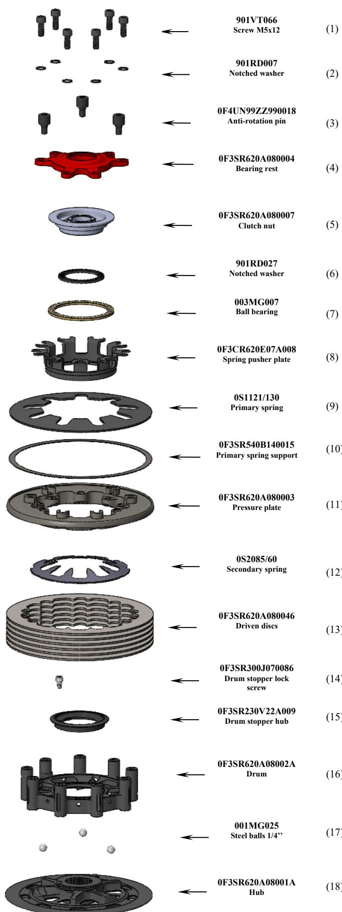
The Drum/Hub group is supplied pre-assembled. **IN CASE OF NEED**, as to check the ramps wear, please see hereinafter the specific procedure to disassemble the STM drum/hub group.
