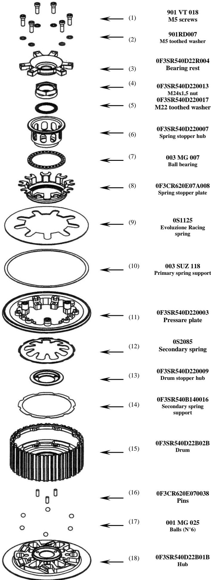
Pre-assemble the hub pack: place the 6 steel balls (17) at the bottom of the grooves of the hub (18) using a small amount of grease then fix the drum (15) onto the hub (18) with an M6x1 screw in an at-rest position.
