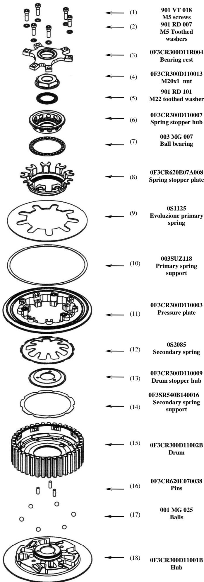
Pre-assemble the hub pack: place the 6 steel balls (17) at the bottom of the grooves of the hub (18) using a small amount of grease then fix the drum (15) onto the hub (18) with an M6x1 screw in an at-rest position.
