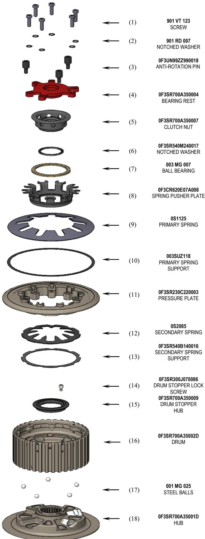
The Drum/Hub group is supplied pre-assembled. **In case of need**, as to check the ramps wear, please see hereinafter the specific procedure to disassemble the Drum/Hub group.
