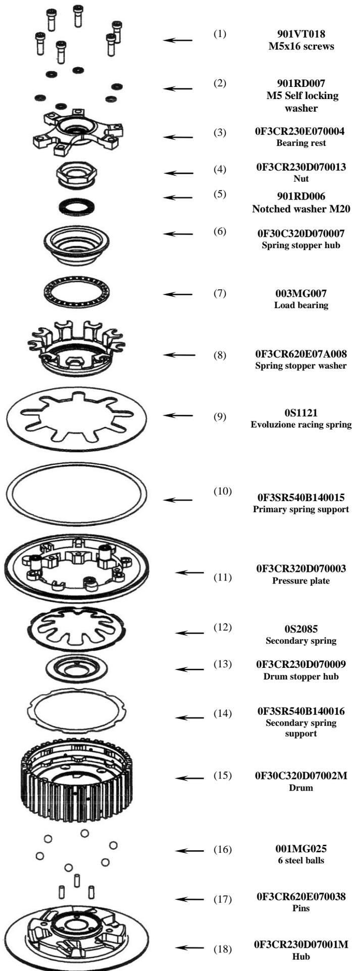
Pre-assemble the hub pack: place at the bottom of the grooves the 6 steel balls (16) onto the hub (18) using a small amount of grease. With an M6 screw fix the clutch drum (15) onto the clutch hub (18) in an at-rest position.
