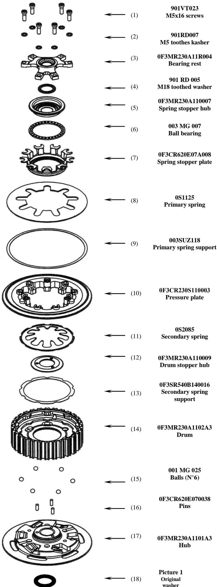
Pre-assemble the hub pack: place the 6 steel balls (15) at the bottom of the grooves of the hub (17) using a small amount of grease then fix the drum (14) onto the hub (17) with an M6x1 screw in an at-rest position.
